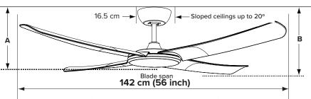
A: 30 cm CEILING TO BOTTOM OF MOTOR **B: 29 cm** CEILING TO BOTTOM OF BLADES
