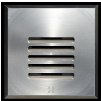
The Step Lite Louvre Square has an 88mm (3 1/2") square flange with a flush surface look with no protrusions. The 45 degree louvre eliminates all upward light making this luminaire ideal for illumination of steps and low level features such as exterior paved areas.
