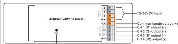
Program Key: short press to switch on/off load, press and hold down to increase/decrease light intensity
