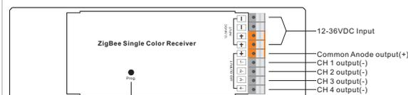
Program Key: short press to switch on/off the device, press and hold down to increase/decrease light intensity
