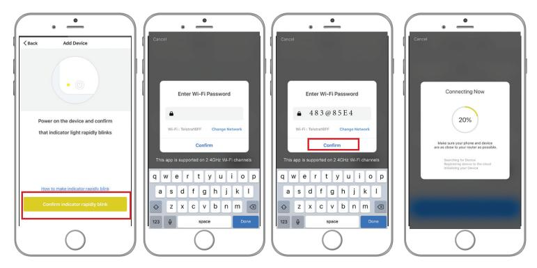
When the indicator light is blinking rapidly (2 times per second) press the confirm indicator rapidly blink button and type in your 2.4 gigahertz home WiFi password then press **'confirm'**.
