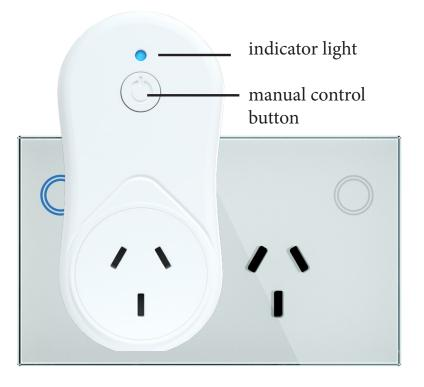
To connect the Smart WiFi Plug to your WiFi press and hold the manual control button for about 5 seconds until you hear a **click**. Let go of the button as soon as you hear the **click**. Then press button once again to activate blinking. **The red indicator light should now blink rapidly (2 times per second).**
