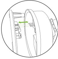
Contacts locate into 3-way terminal block for speedy connection.
