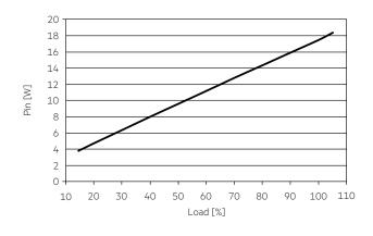
4.1.6 Phase cut dimming curve (depends dimmer)
